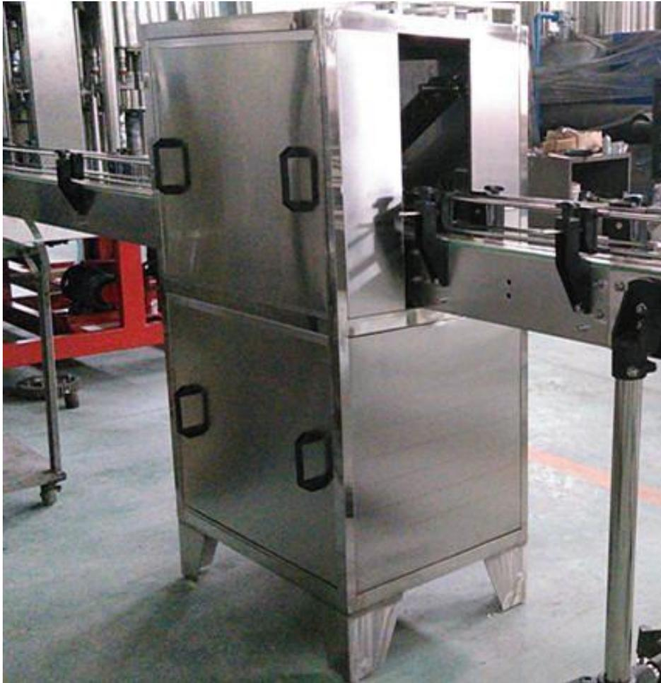
Drying machine is the pressure generated by the vortex air pump air through the air knife hair spike of high-speed wind curtains, drops the bottle blew the body, easy bottle labeling and packing..
